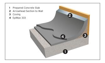
Where required, professional coving can be installed using a trowellable mix of 1 volume of mixed EpiMax 225 and up to 4 volumes of EpiMax EA4. Please note that coving work is rather specialised and may require some site modification to suit the specific site conditions. Allow to cure and then protect with EpiMax 333.
